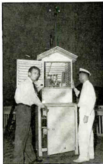
Photo—Science Service Wilbur S. Hinman, Jr., left, radio engineer of the National Bureau of Standards, and C. A. Kelly, chief aerographer of the U.S. Naval Air Station, Anacostia, D. C., watch the self-contained weather observing station observe the storm that is coming. The record untouched by human hands is sent by radio to a distant office. (See photo on cover.)
